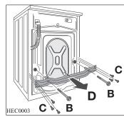
**5.** Remove the bracket **D** and tighten up the six smaller bolts **C**. Slide out the relevant plastic spacer **E**.
